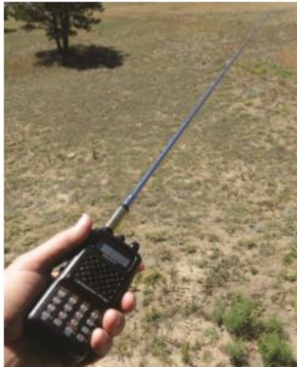
Handheld transceiver with half-wave antenna for 2 meters.
