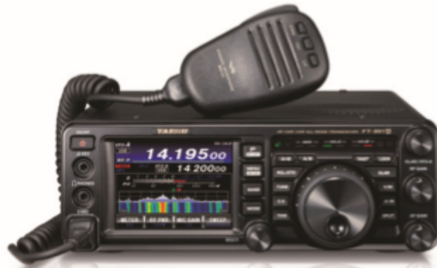
The Yaesu FT-991A is an example of a transceiver that covers HF, VHF and UHF.
