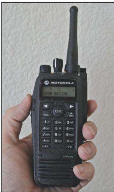
Photo A. The Motorola XPR 6550 is a popular DMR portable radio, available in VHF and UHF models.
