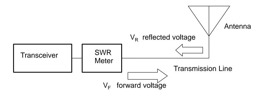
SWR meter is inserted into the transmission line, which usually requires an additional cable between transceiver and SWR meter.
