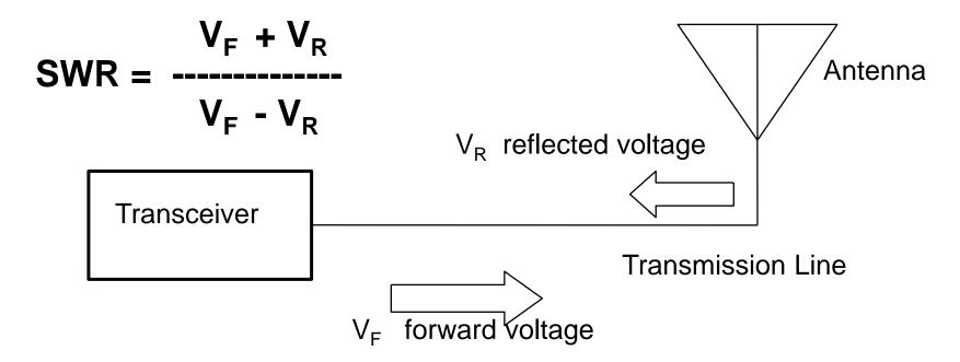
**Perfect Match:**  $V_R = 0$ , no reflection, SWR = 1.0 **Small reflection:**  $V_R = 20\%$  of  $V_F$ , SWR = 1.5 **Large reflection:**  $V_R = 80\%$  of  $V_F$ , SWR = 9 **Open load:**  $V_R = 100\%$  of  $V_F$ , SWR = infinite
