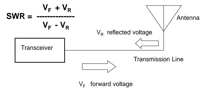
Transceiver, transmission line and antenna are all nominally the same impedance (50 ohms for amateur radio work).
