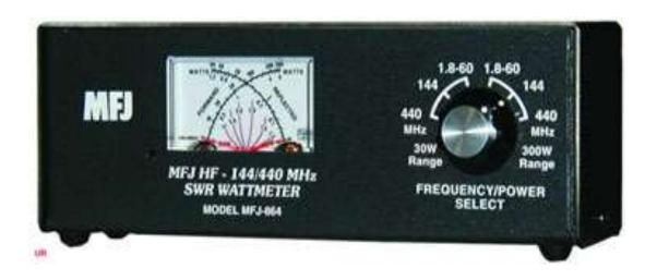
Note the use of the cross-needle meter to avoid the need to "cal" the measurement
