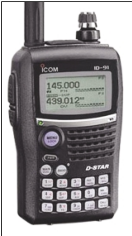
Figure 5. The IC-91AD is a dualband D-STAR handheld transceiver from ICOM. (Photo courtesy of rigpix.com)
